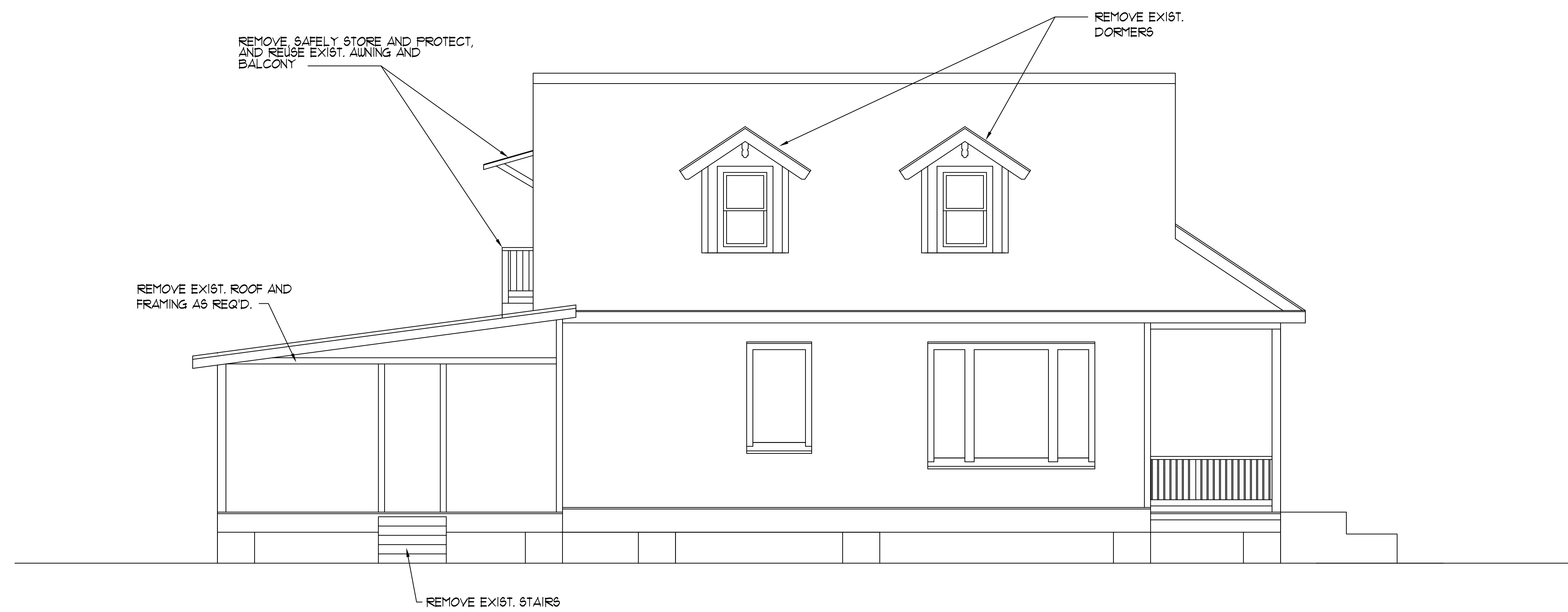
LEFT SIDE ELEVATION DEMOLITION PLAN
